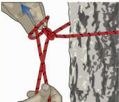
**5** Pinch the working line with your left-hand fingers. Pull it up through the loop to tighten the knot on itself.
