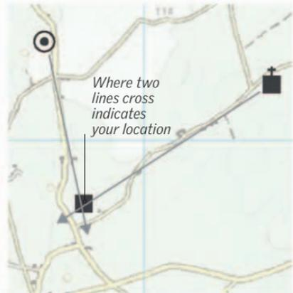
**1** Using your compass, take bearings to the features on the ground.
