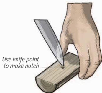
**3** Make the bearing block from hard wood about 3–4in (7.5–10cm) across. Cut it to a length of 4–5in (12–15cm), split it in two, and make a notch in it.
