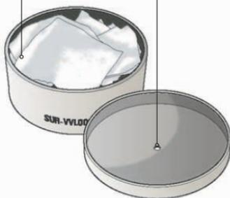
**1** Turn the lid of a can upside-down and hammer a nail into the center. Usually, the smaller the hole, the better.
