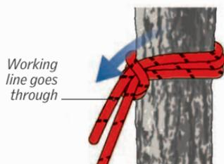
**4** Bringing the working line around, thread it under itself to complete the knot. Lock the knot into position.
