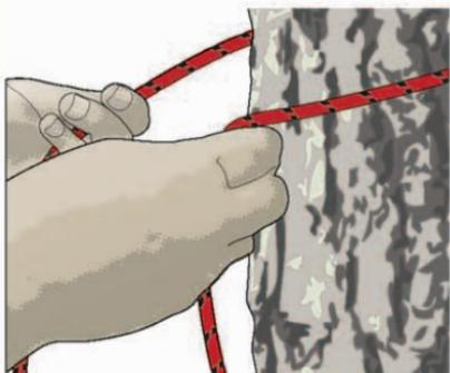
**1** With the working line in your right hand and the standing line in your left, pass the cord around the tree.
