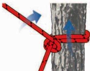
**3** Pass the working end over the top and around the standing line again, and once more around the fixture.
