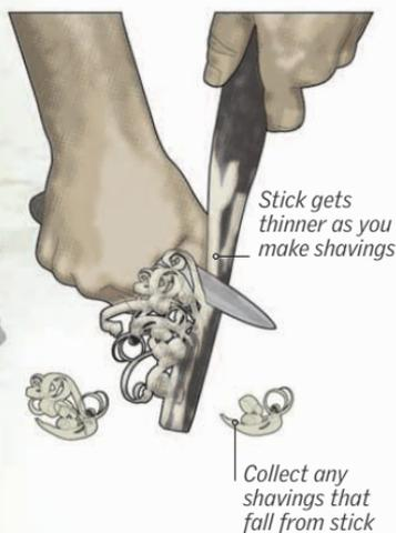
**2** Turn the stick slightly and run the knife down the edge created in step 1 to create a second shaving. Turn the stick again and repeat, working around it.
